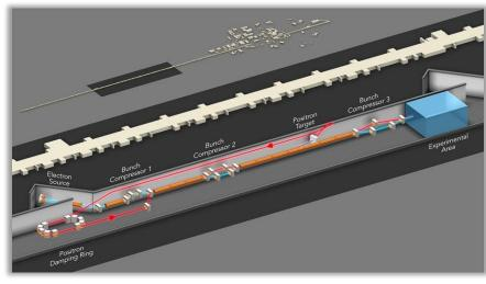
\*E333 experiment planned for filament regime positron PWFA.
